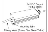
3. **Power Supply:** Identify primary wires, secondary wires, and location of mounting tabs.
