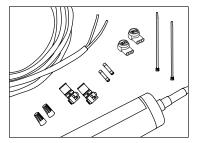
Supplies required: Conduit and electrical enclosure for power supply (if not placed in a sign made from enclosure rated material), #6 or #8 pan head screws, UL Listed PLTC cable, UL Listed electrical wire connectors (e.g., wirenuts), silicone.
