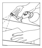
4. Clean Channel Letter: Clean inside the letter with rubbing alcohol and allow to dry.
