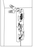
8. Cap all Unused Wires: The strand of modules should not be looped to create a closed circuit.
