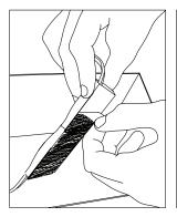
5. Peel and Stick: Using predetermined layout and LED placement from step 3, remove tape backing and stick modules into place. Ensure modules are firmly attached. (CAUTION: when handling the module, avoid pressing down directly on top of LED.)
