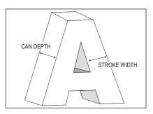
3. Layout: Noting can depth, stroke width and face material, use layout guidelines and power supply capacity charts on page 2 to determine spacing and amount of LEDs required.
