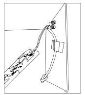
**Connect Power Supply to First** Module on String: See Power Supply Install Guide for more information regarding power supply installation.
