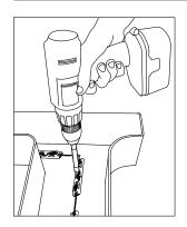
6. Fasteners: If desired. modules can be secured with #6 pan head sheet metal screws or 1/8 in (3 mm) aluminum rivets.
