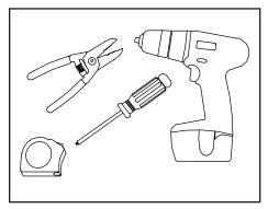
Tools required: Measuring tape, wire strippers. Optional: Drill, screwdriver.
