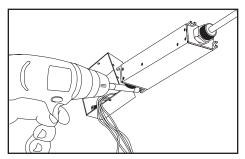
6. Units may be mounted in any orientation using mounting tabs.
