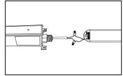
Connect modules to power supply: Using UL Listed electrical connectors, daisy chain PosterBOX modules as required and connect to power supply. Modules may be daisy chained in series or parallel configurations.
