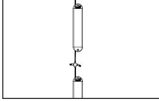
Connect modules: Each module has 2 ft (0.6 m) of wiring on each side. Cut wires as needed leaving enough to connect the modules. Modules may be connected in series or parallel.
