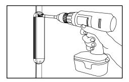
Fasteners: If desired, modules can be secured using #8 (M4) pan head sheet metal screws or 5/32" (4 mm) aluminum rivets.
