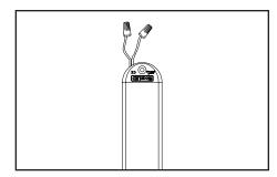
Cap all unused wires: The strand of modules should not be looped to create a closed circuit.
