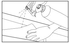
Clean sign box: Using a non-oil based cleaner, clean the inside surface of the sign. Be sure to clean any mounting surfaces with alcohol for proper tape adhesion.
