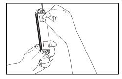
Peel and stick: Using provided double stick tape, mount PosterBOX modules to sides of sign box. For best performance it is recommended that the modules be mounted flush against the rear wall of the sign box.
