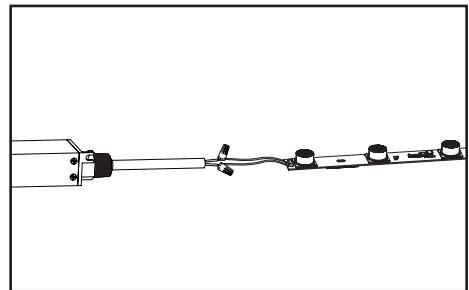
7. **Connect to power supply:** Using UL Listed electrical connectors, daisy chain product as required and connect to power supply.
