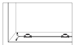
Fasteners: If desired, modules can be secured to sides of sign box using #6 (M3) pan head sheet metal screws or 1/8" (3 mm) aluminum rivets.
