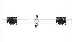
Connections: Modules may be connected in series or parallel. Modules should not be looped to create a closed circuit. Cap all unused, exposed wire ends.
