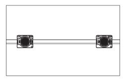
**NOTE:** For optimum internal reflection in single-sided sign boxes, mount modules 0.2"-0.4" (5-10 mm) from rear wall. For double-sided sign boxes, mount modules in center of return.
