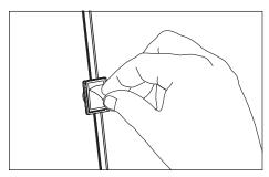
Peel and stick: Using provided double stick tape, mount PosterBOX Mini modules to sides of sign box.
