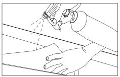
Clean surface: Clean inside of sign box with rubbing alcohol and allow to dry. Clean all mounting surfaces with alcohol for proper tape adhesion.
