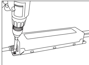
**4. Mount Power Supplies:** Use mounting tab in corner to secure power supply.
