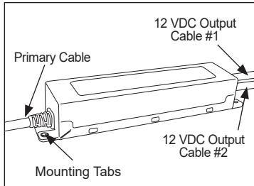
**3. Power Supply:** Identify primary cable, 12 VDC output cables #1 and #2, and location of mounting tabs.
