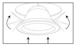
Push springs clips to vertical and slide luminaire into circular opening in ceiling.
