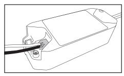
2. Push primary wiring into N and L terminals on primary side push-in connector.
