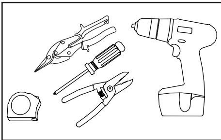
**Tools required:** Measuring tape, wire strippers, sheet metal shears/snips (if cutting product), drill, and screwdriver.
