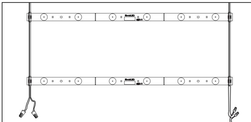
4. **Connections:** LED Strips may be connected in series or parallel, using appropriate UL/CE Listed wire connectors. Cap all unused wires. Connect power supply output to first LED strip on string. See power supply install guide for more information regarding power supply installation.
