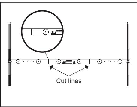
2. **Adjustment of width (Long):** If a narrower width is required, use a pair of sharp sheet metal shears/snips to cut along cut lines. Deburr end of cut product with metal file or sandpaper to prevent electrical shorts.
