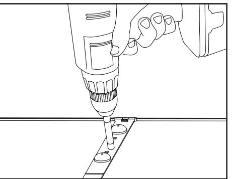
3. **Fasteners:** Use fasteners or silicone as necessary to fix LED strips into place. Refer to components list above for acceptable fasteners.
