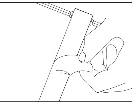
1. **Peel and stick:** Clean inside sign with rubbing alcohol and allow to dry. Using predetermined layout and LED placement from previous step, remove tape backing and stick LED strips into place. Ensure strips are firmly attached.
