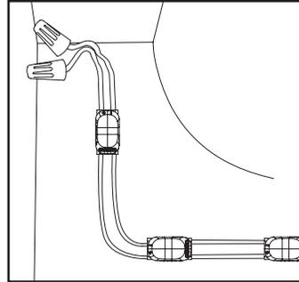
7. **Cap all unused wires:** Using appropriate UL Listed wire connectors (refer to components list on page 1), cap all unused wires. Strand of modules should not be looped to create a closed circuit.
