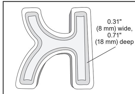
1b. **Preparing block:** Mill 0.31" (8 mm) wide channel an additional 0.28" (7 mm) down (0.71" [18 mm] total) to improve light transmission around edges.
