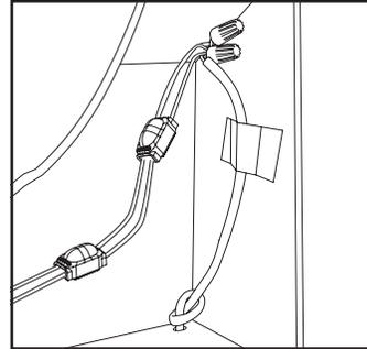
8. **Connect power supply to first module on string:** See power supply install guide for more information regarding power supply installation.
