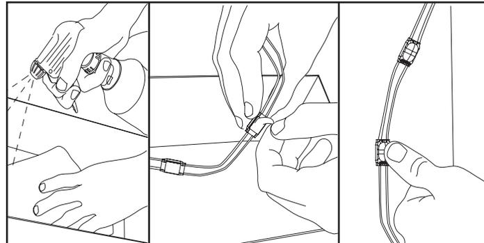
4. **Peel and stick:** Clean inside sign with rubbing alcohol and allow to dry. Using predetermined layout and LED placement from Step 3, remove tape backing and stick modules into place. Ensure modules are firmly attached. **NOTE:** If installing in a narrow channel, tape may be unnecessary. Other means of securing strip (sealant, vinyl, etc.) are also acceptable.
