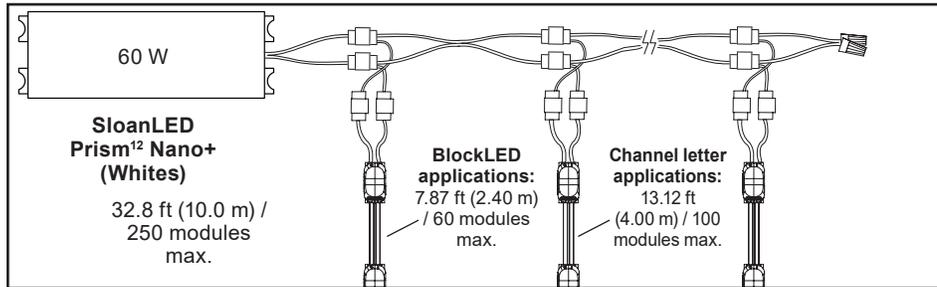
**NOTE:** It is recommended to connect no more than the following in series to minimize line loss:
