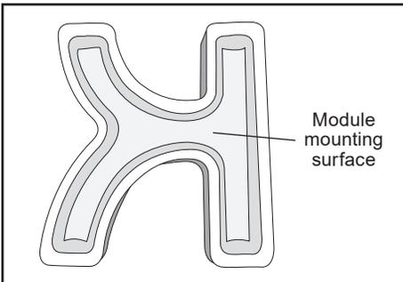
1a. **Preparing block:** It is recommended to mill down module mounting surface 0.43" (11 mm), giving 0.08" - 0.12" (2-3 mm) space between lens and back tray.
