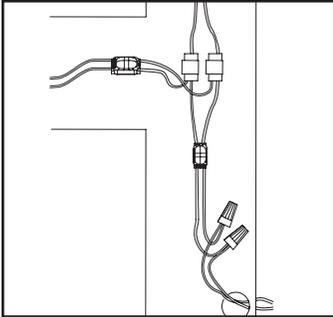
6. **Connections:** Modules may be connected in series or parallel. **Tip:** Discarding a module can allow longer wire lengths for connections.
