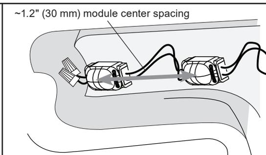
2. **Module placement:** Mount modules ~1.2" (30 mm) apart (center-to-center) using provided tape, or silicone as necessary. **NOTE:** Avoid silicone on top of lenses.
