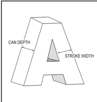
3. **Layout:** To populate sign, refer to SloanLED Prism<sup>12</sup> Nano+ density guidelines as well as power supply loading chart (page 4) to determine appropriate number of modules and power supplies.
