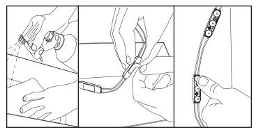
4. Peel and stick: Clean inside sign with rubbing alcohol and allow to dry. Using predetermined layout and LED placement from Step 3, remove tape backing and stick modules into place. Ensure modules are firmly attached.
