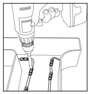
Fasteners: Use fasteners or silicone as necessary to fix modules in place. Refer to components list above for acceptable fasteners.
