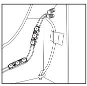
Connect power supply to first module on string: See power supply install guide for more information regarding power supply installation.
