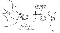
1. Connect overmold connectors: Align arrow on male connector to arrow on female connector and push connectors together until fully seated.
