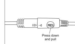
2. Disconnect overmold connectors: With thumb, press down the "Press" on the female connector and pull on male connector.
